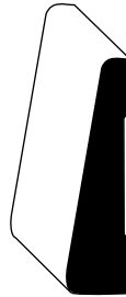
BEVEL 158 5/8" x 1-5/8" | (SP) (FJ) (FJP) x 324 5/8" x 2-1/4" | (SP) x (FJ) x (FJP) x (M) 158 9/16" x 1-9/16" | (M) x
