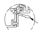
DETAIL D SCALE 1 / 2 HP INTERIOR SILL ADAPTER INCLUDED WITH ALL INSWING DOORS; OPTIONAL WITH OUTSWING DOORS.
